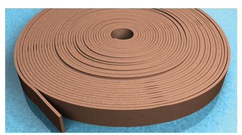
IPM-TEK produces Proprietary, Tight Tolerance, PTFE Bearing Tape that is designed to eliminate scoring, in hydraulic and pneumatic cylinder applications, by preventing metal to metal contact. Our Bronze Filled PTFE compound provides excellent light-duty, low friction performance.
